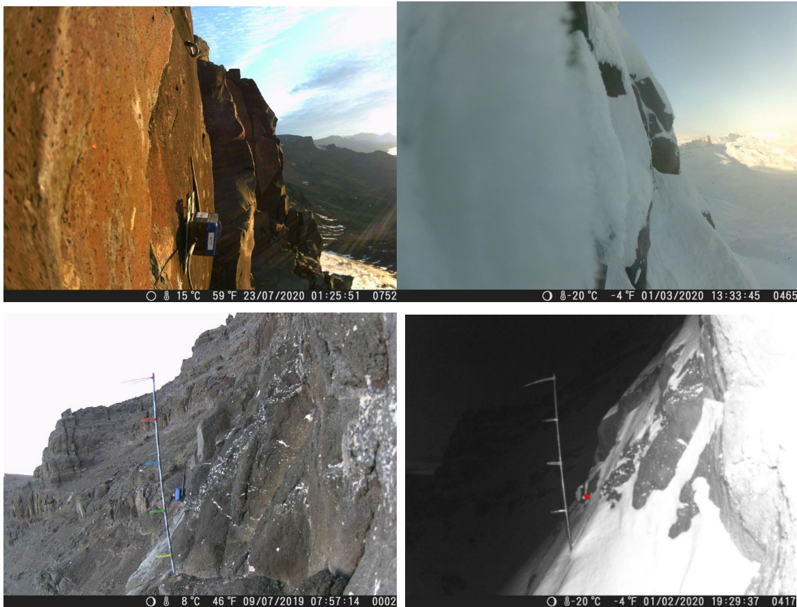
Figure 11: Time lapse images showing snow encrusting a vertical rock wall (top, A53AE5 thermistor string) and the effect of a small ledge on accumulating more snow (bottom, A53AED thermistor string).
